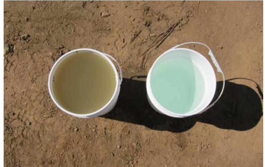
*A research project has shown that tailings water can be treated with coke, a byproduct of our process which is almost pure carbon. The treatment is similar to using a home water filter. Pictured here, tailings water before (left) and after (right) coke filtration.*
