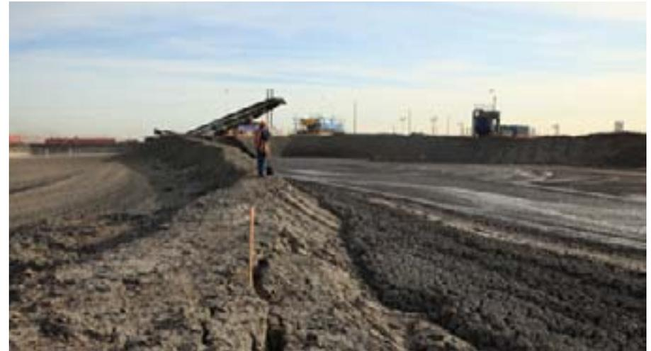
*A commercial-scale demonstration of using centrifuges to dewater fluid fine tailings will begin operations in 2012.*
